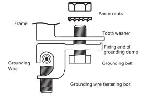
Figure 11 Clamp Grounding Method Note: TYCO. 1954381-1 (Recommended) is used in figures above.
