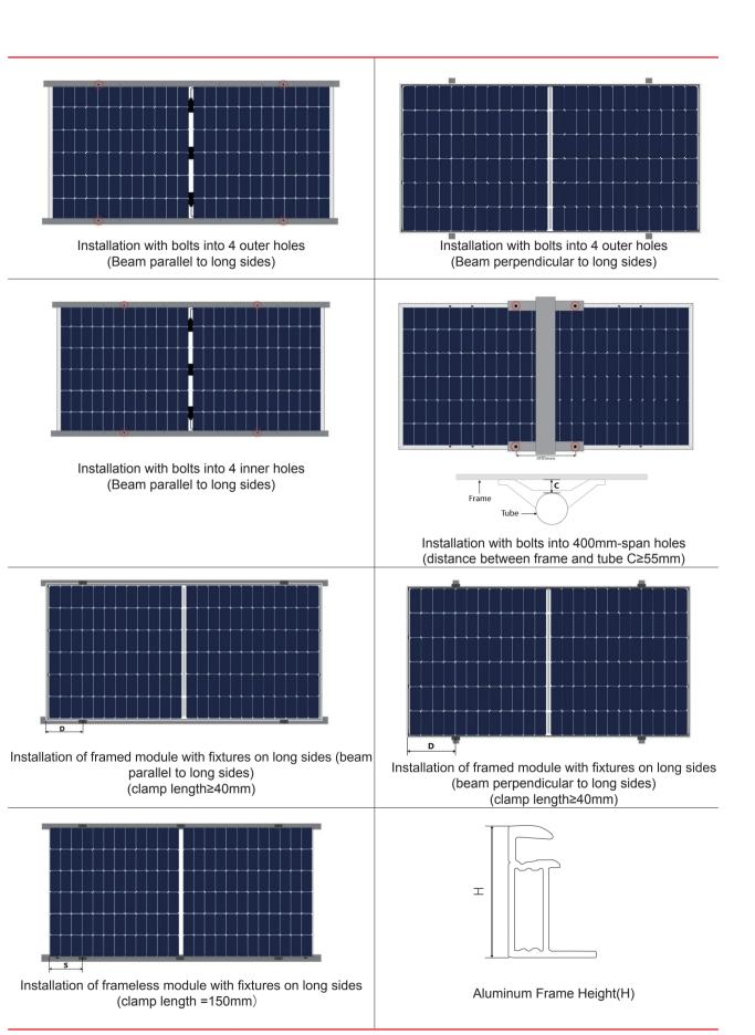
Figure 9 Bifacial Module Installation Annex
