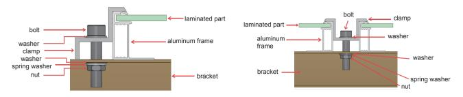
Figure 5 Clamp Installation of Monofacial Module
