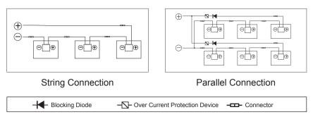
Figure 10 Series Connection and Parallel Connection Circuit Diagram
