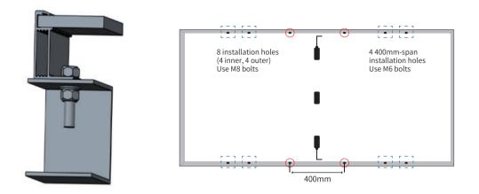
Figure 4 Bolt Installation of Monofacial Module
